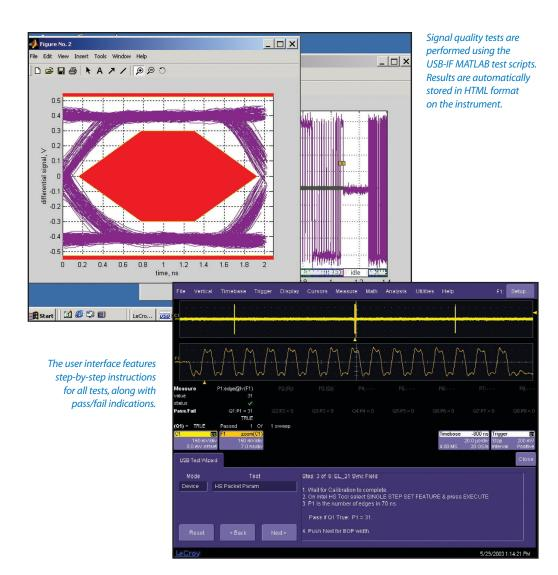
The USB2 Test Package is a software option for LeCroy WaveMaster, SDA, and WavePro 7300 instruments. The package provides a complete acquisition and analysis system for USB 2.0 devices, hosts, and hubs, as specified in the USB-IF USB 2.0 Electrical Test Specification, version 1.0.
